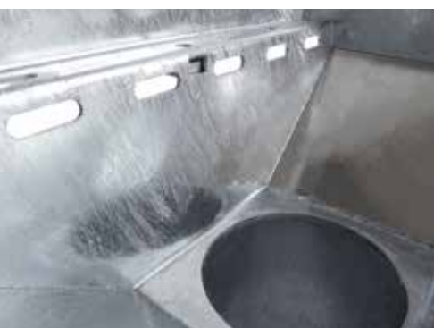
WATER DRAINAGE SLOTS The sump unit's bucket is slotted on both sides for enhanced water run-off deriving from the use of draining asphalt.
